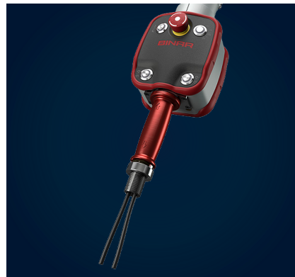
PLUG AND PLAY PNEUMATIC solution for controlling clamping end effectors.
