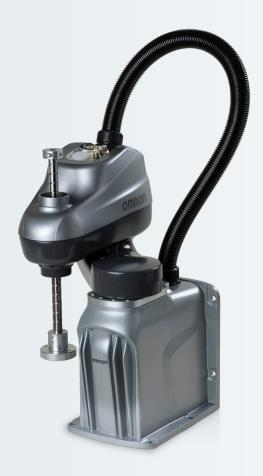
The i4L is a compact SCARA (Selective Compliance Assembly Robot Arm) robot that offers strong performance, a flexible design that makes it simple to install and easy to use features that help maximize productivity.
