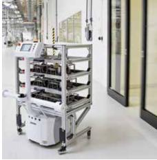
Omron AMRs can interact with facility doors, elevators, and machine equipment
