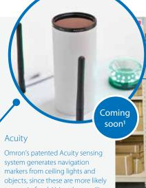
Omron's patented Acuity sensing system generates navigation markers from ceiling lights and objects, since these are more likely to remain fixed. Using these ceiling features along with the standard floor level map, the system can identify the robot's position no matter how frequently the environment on the floor changes.
