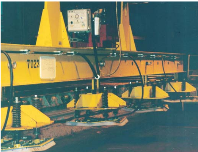
Hi-temperature vacuum lifter for moving hot aluminum from the rolling line to the cooling stack.
