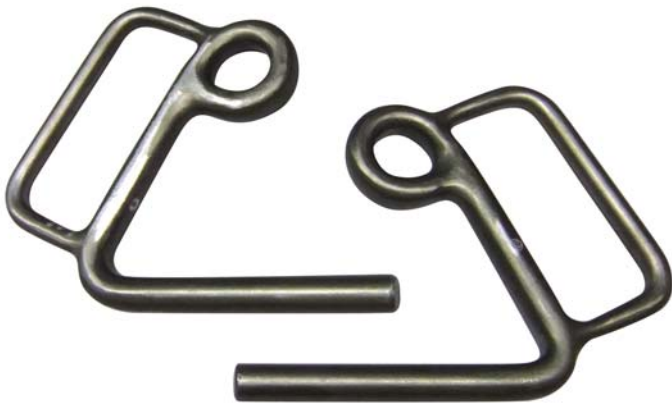
3/4" diameter L-Hooks with 6-1/4" reach, special 6" foot on hook, handle on the back, and a 250 pound working load limit at a specific angle.
