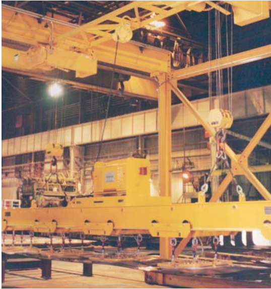
Heavy duty vacuum lifter with vacuum pads mounted on wheeled trolleys for ease of pad adjustment.
