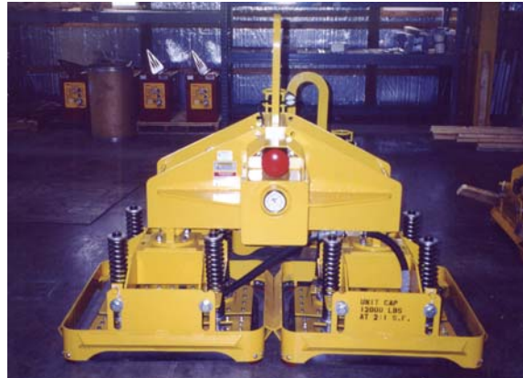
Auto-attach/release bail on this vacuum lifter allows for hands-free operation. Available as 6,000 pounds single pad or 12,000 pound dual pad units, these 33" square pads are designed for handling material in steel and aluminum mills.
