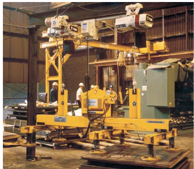
This six-pad vacuum lifter, dedicated to a finish shear, has high twin bails for added stability.
