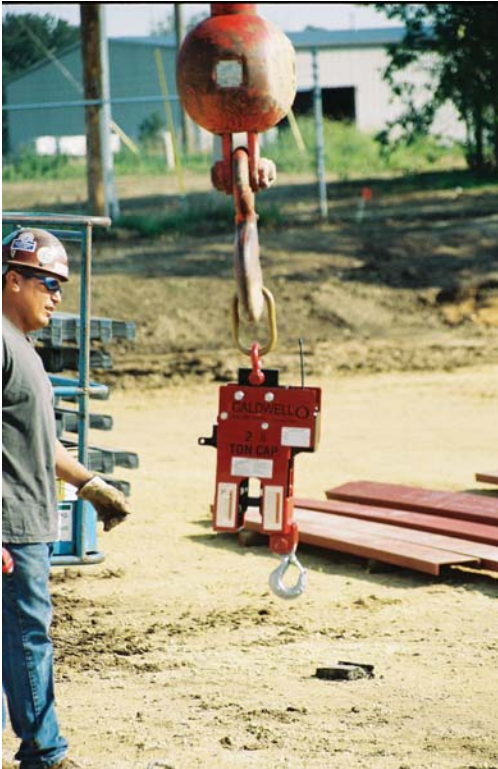
2.5 ton Rig-Release® Hook ready to be rigged
