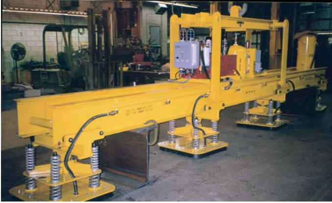
Submersible vacuum lifter can pick and place aircraft aluminum plate from under water in an ultrasonic testing tank.
