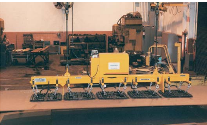
Radio controlled, 20,000 pound capacity unit for loading a burn table for a major steel producer.
