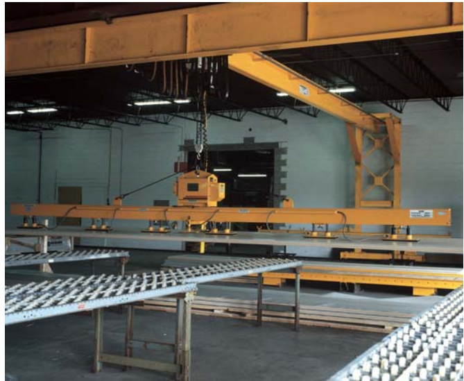
Vacuum unit with rectangular vacuum pads for long narrow steel plate applications.
