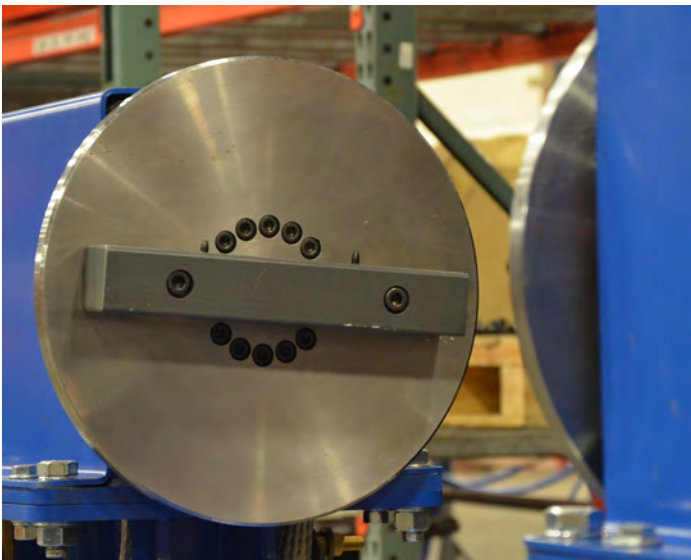
Image: Mounting plate on the Electric Head and Tailstock
