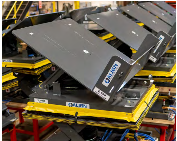
Image: Non-invasive tilt bolted on to a pneumatic lift
