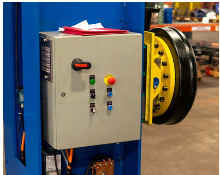
Image: Control Panel for Head & Tailstock Welding Positioners
