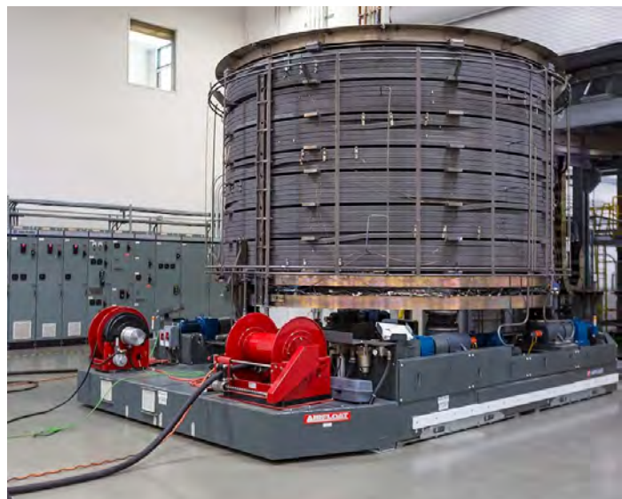
Image: 400,000 lb. Capacity Air Caster Transporter
