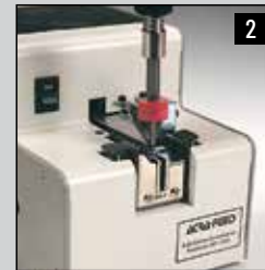
2 Address screw with magnetized bit.
