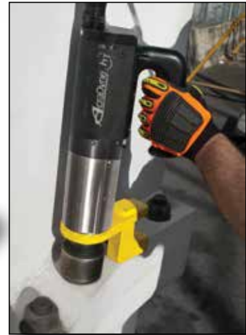
2,800 Nm Torque AEP4W872800B
